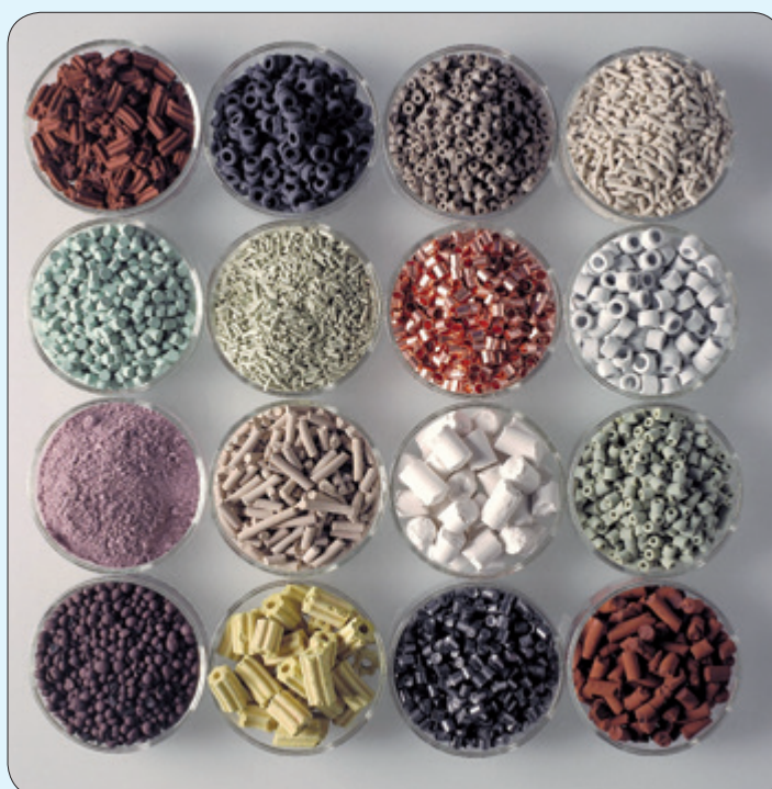
Fig. 5: Examples of solid catalysts in the form of shaped catalyst bodies as applied on an industrial scale (source: BASF SE).
